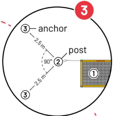
To obtain the ideal position for the sand anchors, unfold the net completely (1). The loops of the top cable mark the positions of the net posts (2). Knock the anchors into the ground at a distance of approx. 2,5 m from the post position (3) with an approx. 90° angle.
