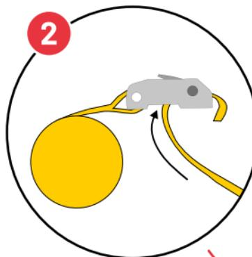
Put the two parts of the yellow straps together as shown. Make sure the loops are positioned at the end of the straps and not near the metal clip lock. Slip the small loops over the sand anchors.
