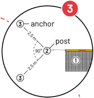
To obtain the ideal position for the sand anchors, unfold the net completely (1). The loops of the top cable mark the positions of the net posts (2). Knock the anchors into the ground at a distance of approx. 2,5 m from the post position (3) with an approx. 90° angle.
