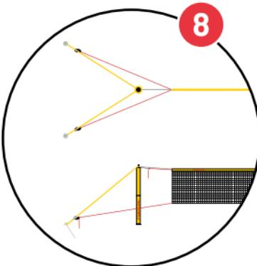
The net tension and net height can be altered to achieve the perfect net by adjusting the tension of the red ropes at the bottom corners of the net.
