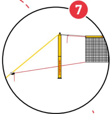
Tighten the yellow straps and adjust the position of the post to set them up vertically. The net should now align midway between the poles automatically. Adjust the lower red ropes to length at the black hook end and attach them to the metal clip locks on the yellow tension straps.
