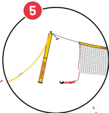
Put the large loops of the tensioning straps and the loops of the net tensioning rope over the top of the net posts and set them up at an angle towards the playing field.
